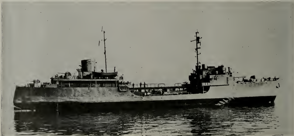
One of a fleet of 23 A. O. G.-type Navy oil tankers powered by diesel engines made by the Cleveland Diesel Engine Division of General Motors. Most of these tankers have four 16-cylinder engines totaling 6400 aggregate brake horsepower.
